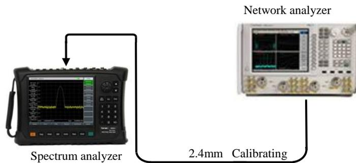
Fig. 12-18 Voltage Standing Wave Ratio Test of Input Port
