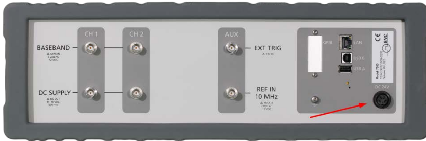
Figure 6: 7000 Series power connector
